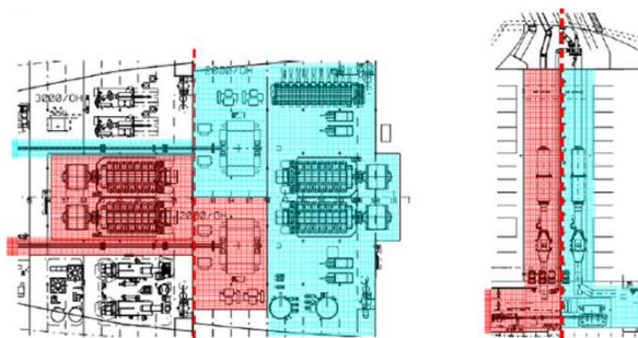
Propulsion / EL production & Distribution – Principles for segregation of the systems
